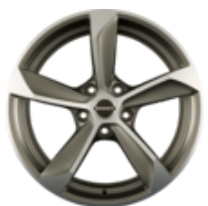
Carex* Alloy Wheel 18" Borbet S, 5-spoke-design, Graphite Polished matt 8 x 18", offset 45 – For tyres 235/40 R18
